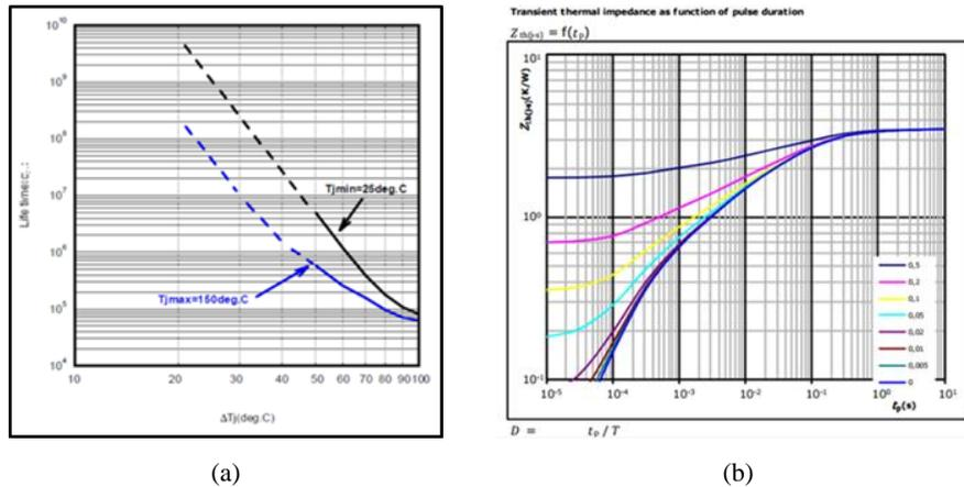
**Fig. 10.** (a) Power cycling lifetime curve, (b) Transient thermal impedance as function of pulse duration.
