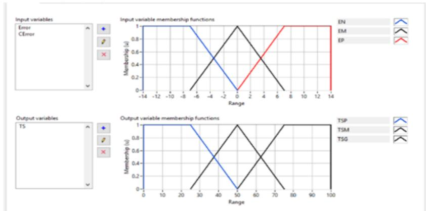
Fig. 8. Input-output membership functions.
