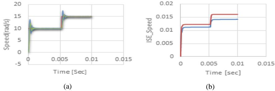
**Fig. 11.** (a) Speed response: proportional control (blue), Fuzzy logic controller (green), and set point (red); (b) Controller index Integral Square Error (ISE), proportional (red), Fuzzy logic (blue).
