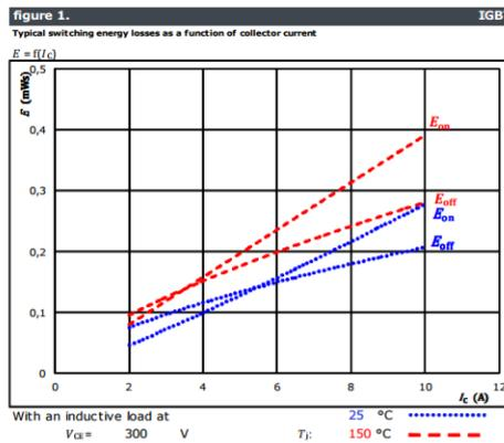
Fig. 3. Typical switching energy losses as a function of collector current.
